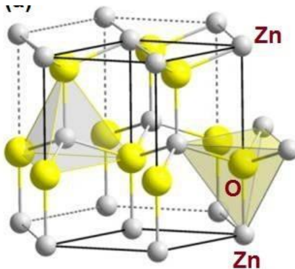
Figure 1-2 : Crystal Structure of ZnO
