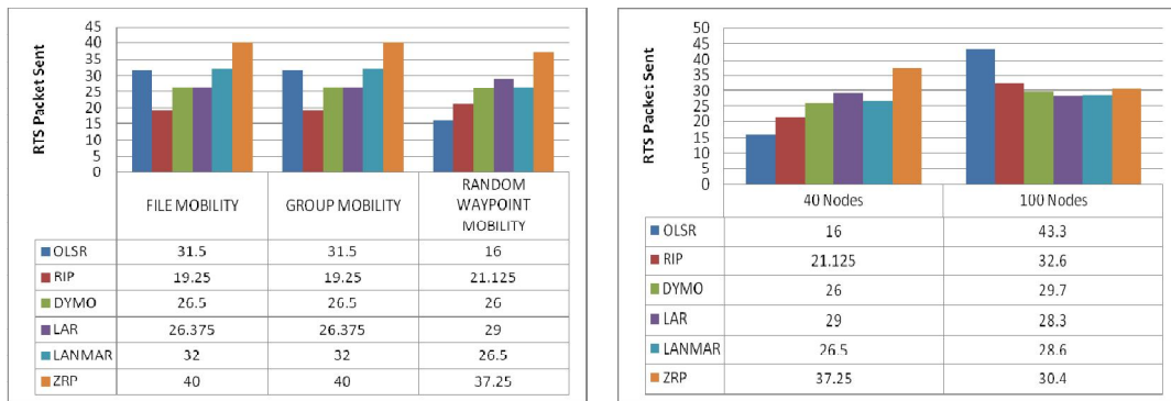
Fig. 4.10(a) RTS Packet Sent vs Mobility Fig. 4.10(b) RTS Packet Sent vs No. of Model Nodes
