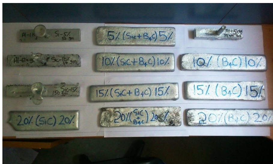
Figure 3.8 – Composite samples fabricated through stir casting
