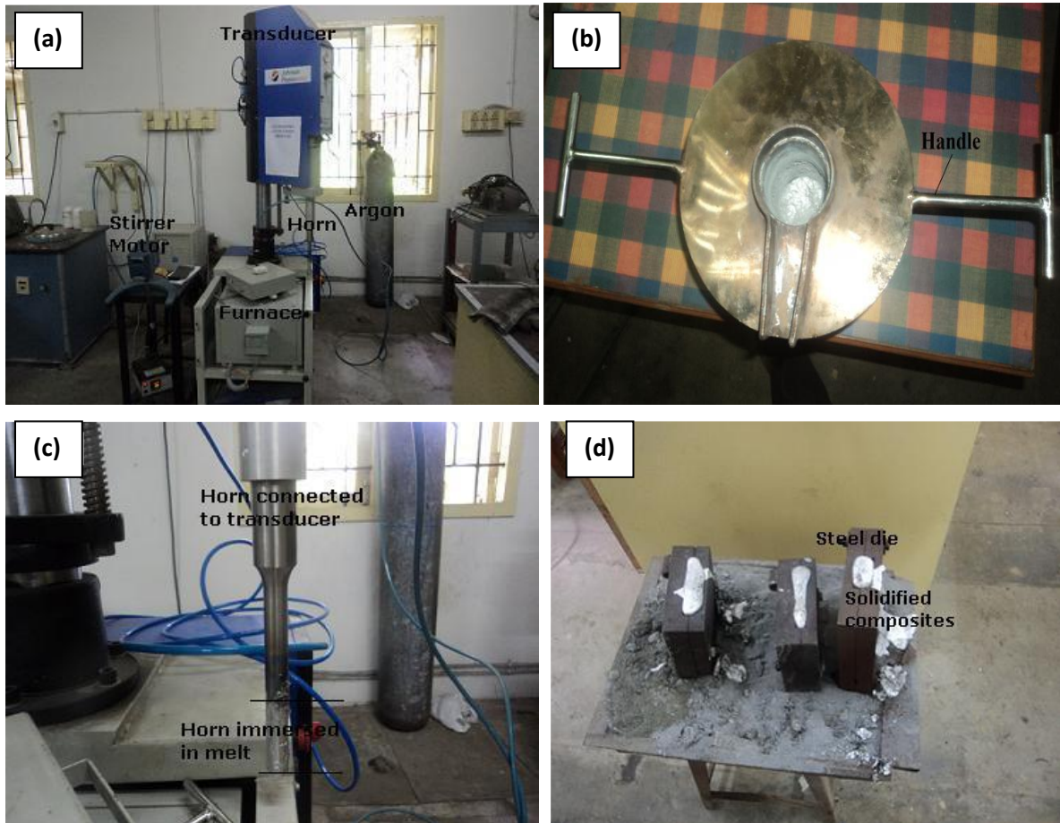
Figure 2.9 (a-d) – (a) Experimental setup, (b) SS crucible, (c) Ultrasonic horn and (d) Solidified composites (Poovazhagan et al., 2013)
