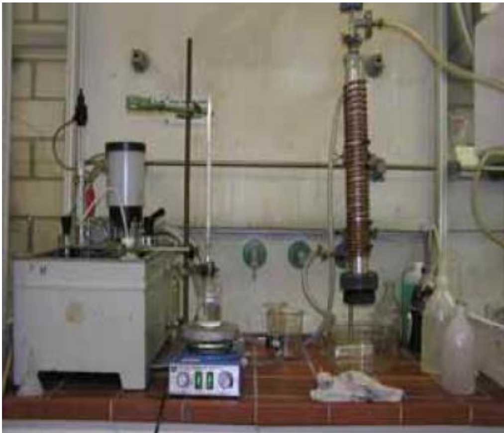
Figure 2.3 - Device used for pumping operation of reagents through ceramic preforms (Dobrzanski et al., 2007)
