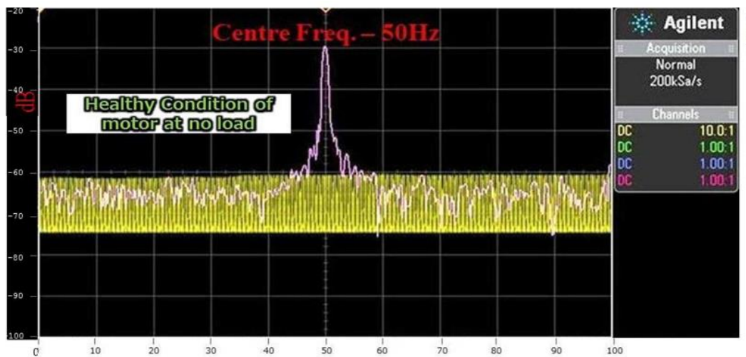
Figure 6.1 SEW EURO DRIVE Motor Spectrum in healthy condition at no broken rotor with no load
