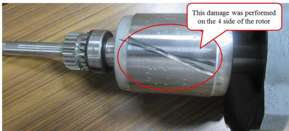
Figure 6.2 Assembly of Broken Rotor Bar
