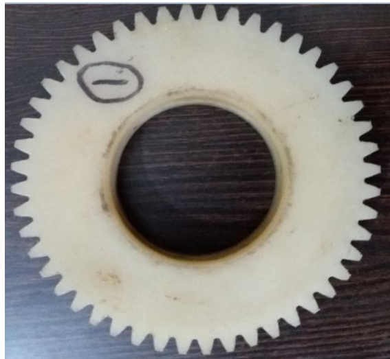
Figure 3.5 Finished GFRP Spur gear
