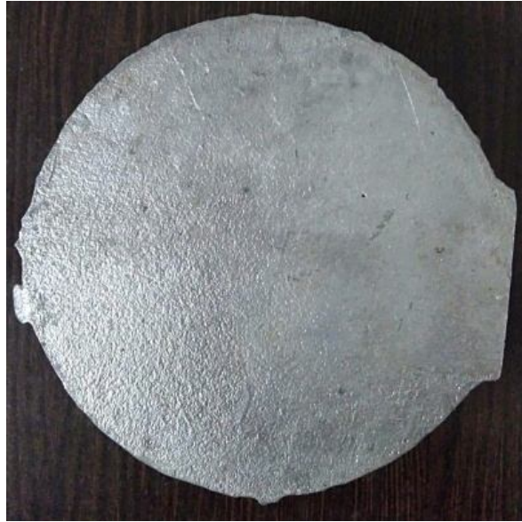
Figure 3.3 MMC blank after stir casting
