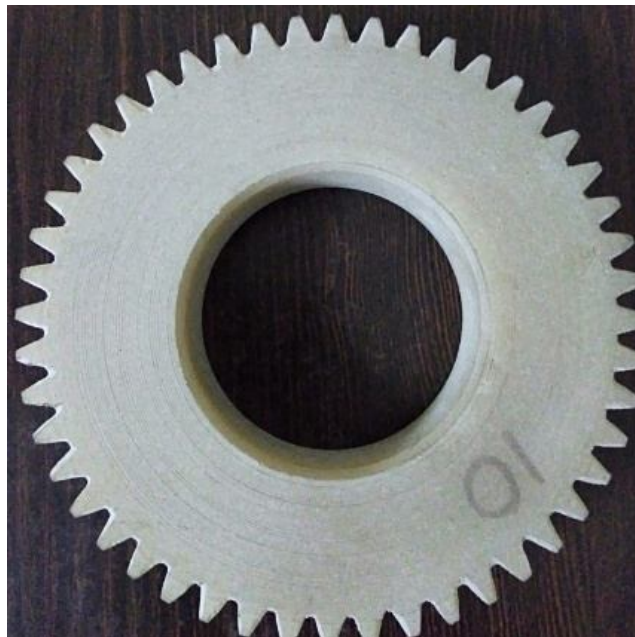
Figure 7.19 GFRP gear after sand blasting
