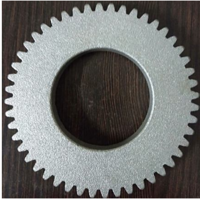
Figure 7.18 MMC gear after shot peening
