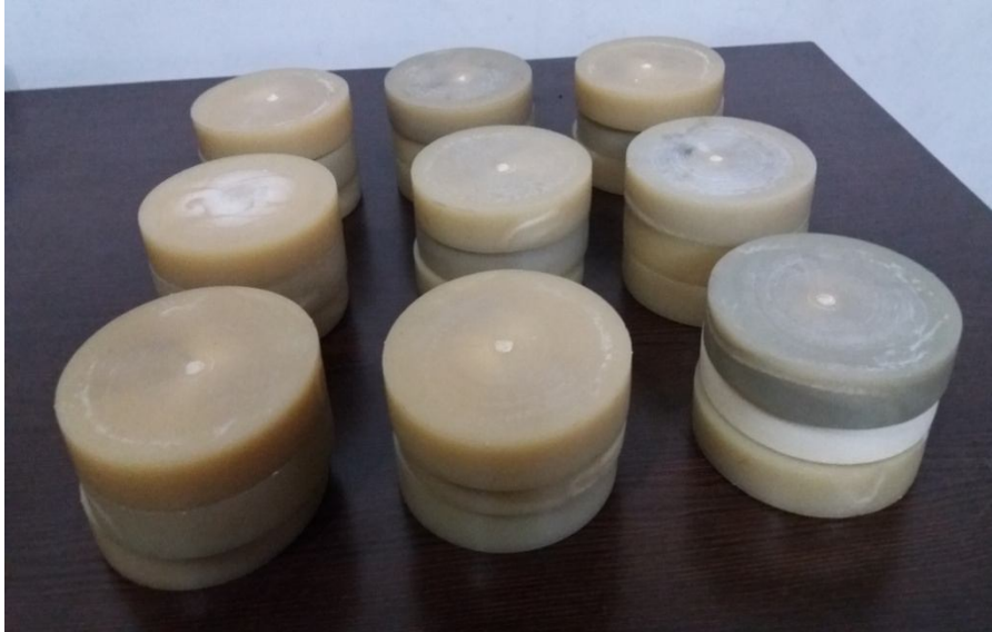
Figure 3.2 Gear blank after injection molding
