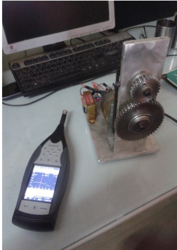
Figure 7.1 Noise measurement setup
