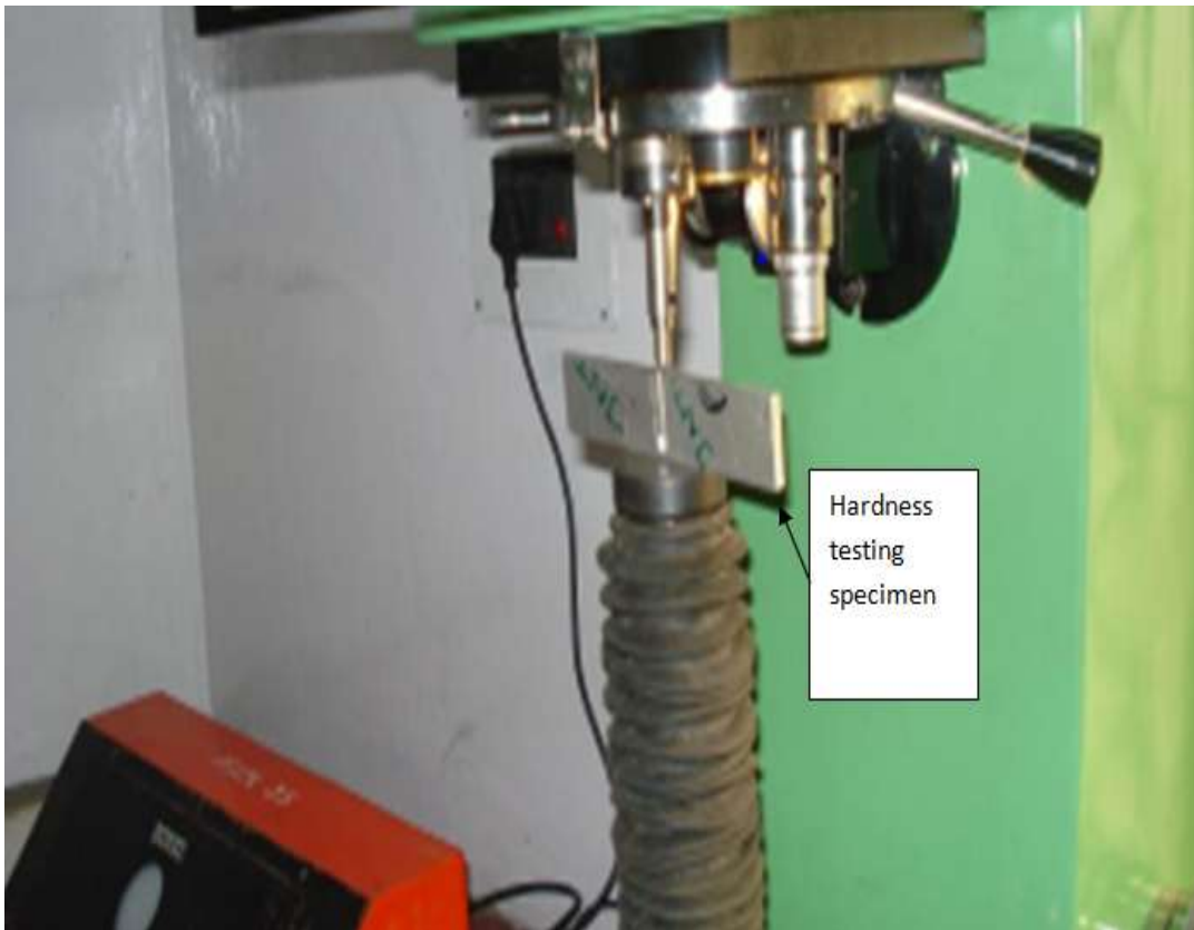
Figure 4.8 Photographic view of Vicker Hardness Testing System
