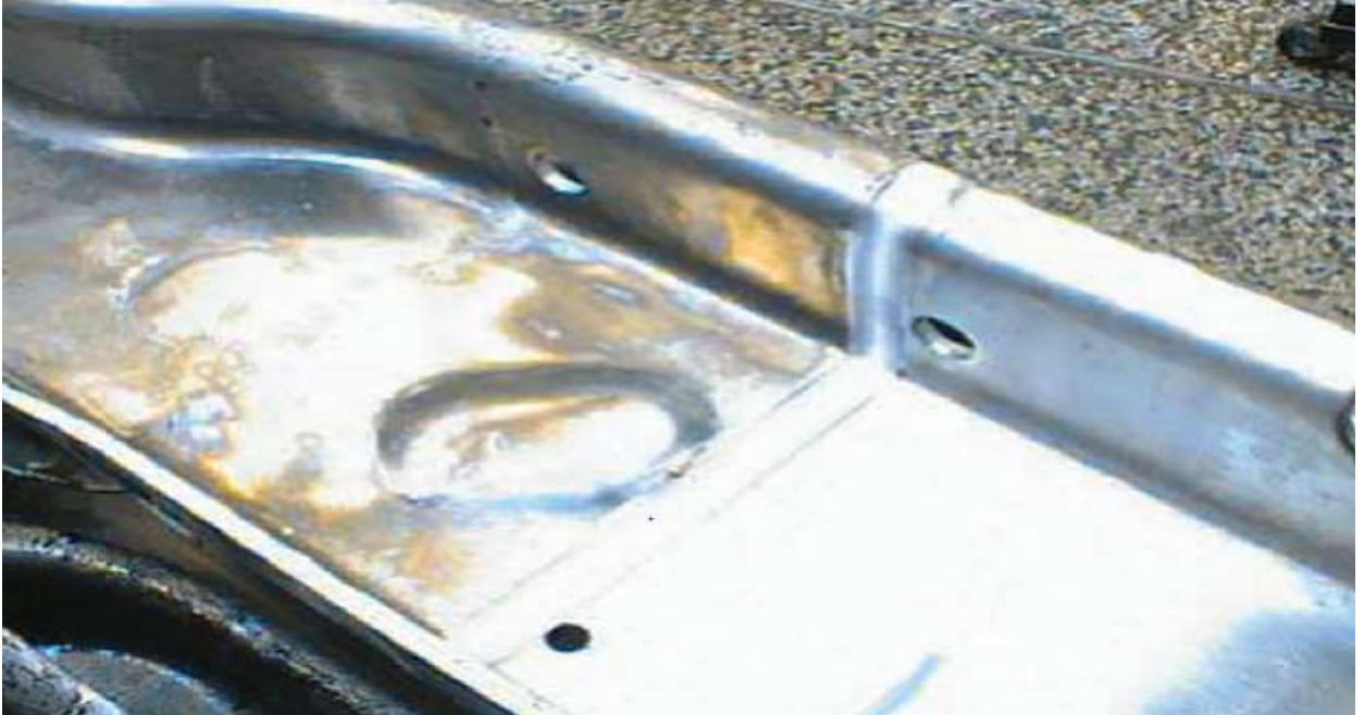
Figure 1.5 Tailor welded blank (Audi B pillar structure) ( http://en.wikipedia.org )
