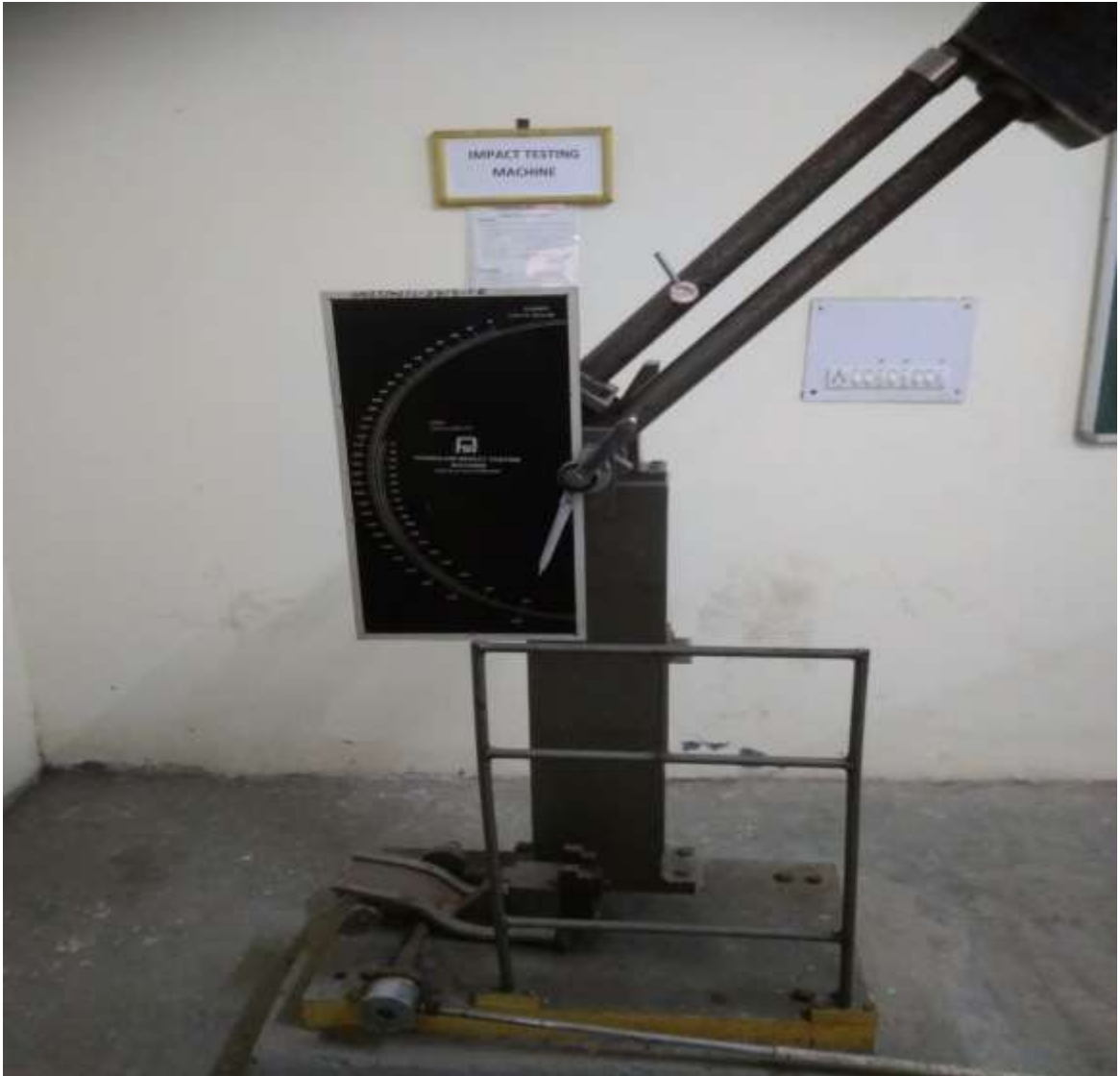
Figure 4.7 Photographic view of Charpy Impact Testing machine
