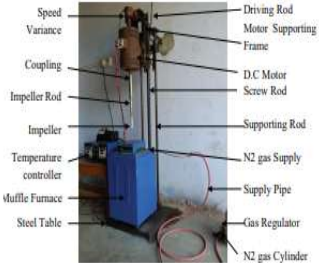
Figure 3.4 Experimental Set-up of Stir Casting
