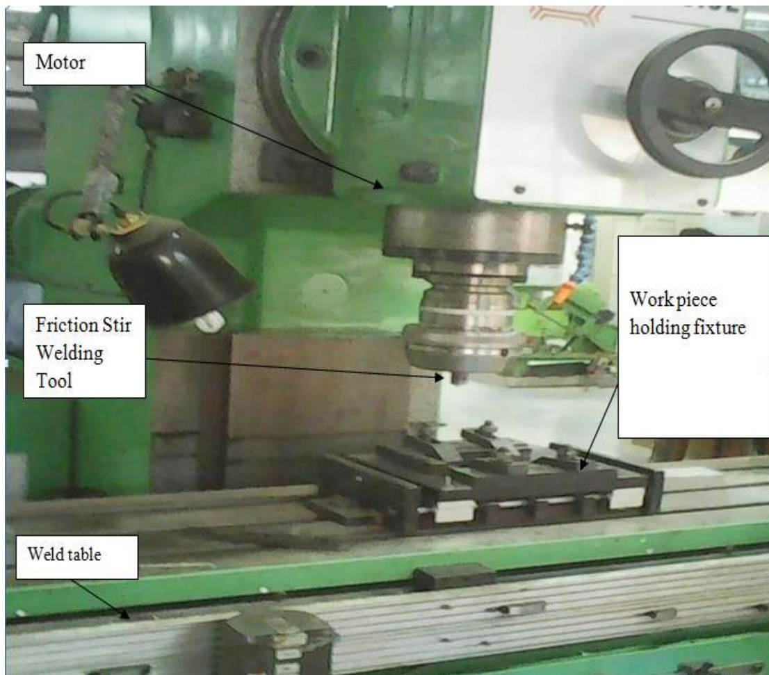
Figure 3.11 Friction stir welding Set-up
