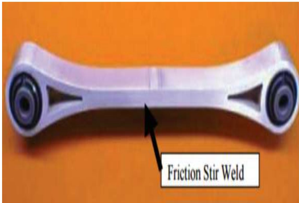
Figure 1.4 Friction stir welded vehicle aluminium link arm ( http://en.wikipedia.org )
