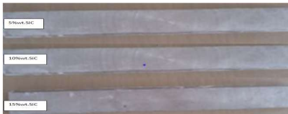
Figure 3.5 Fabricated composite with 5%,10% and 15% SiC Particulates
