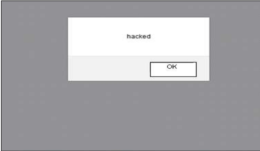
Figure5.26.Output showing vulnerability to XSS attack
