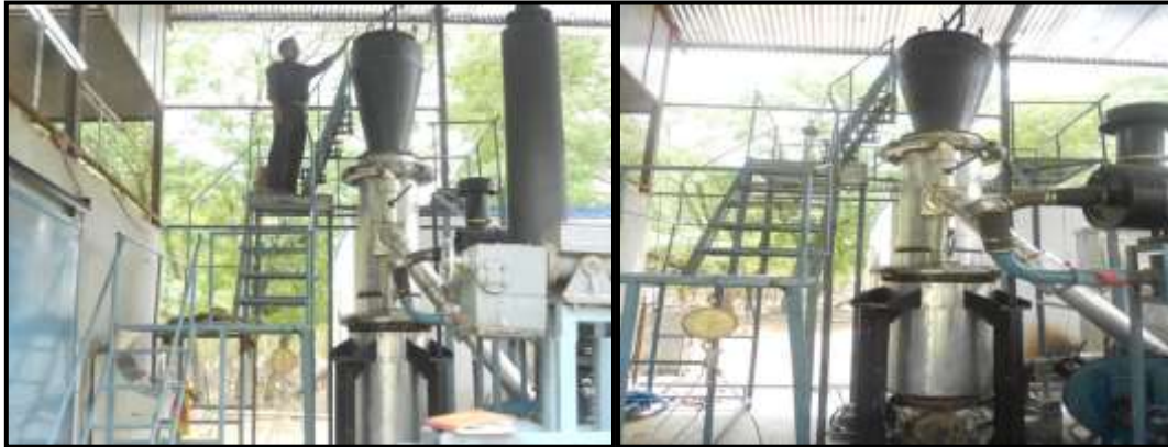
Photograph 4.2 Pictorial Views of double ignition downdraft gasifier
