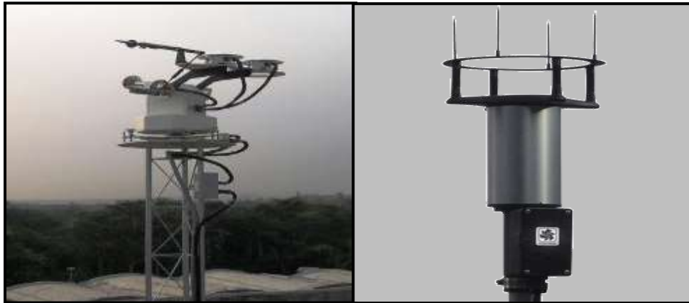
Photograph 4.14 Set up view of pyr heliometer with pyranometer and ultrasonic anemometer
