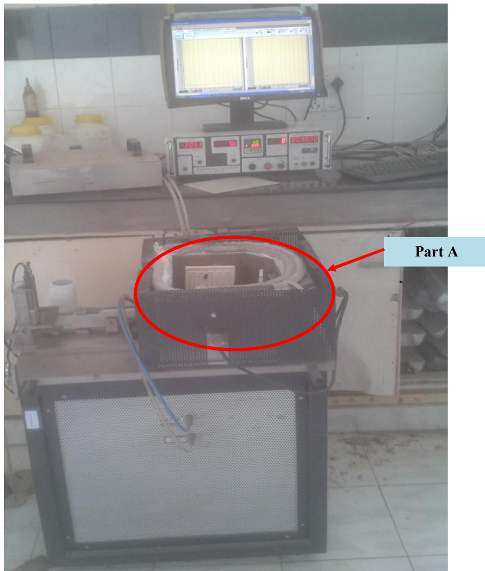
Figure 3.5: Wear Test Rig (TR-20, Ducom, Bangalore)
