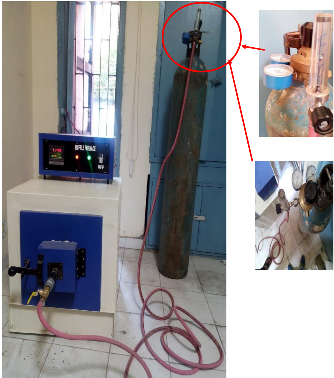
Figure 3.4: Furnace with Inert gas Arrangement
