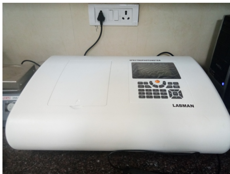
Figure 3.1: Actual photograph of UV visible double beam spectrophotometer (LMSP-UV 1900S, Labman Scientific)
