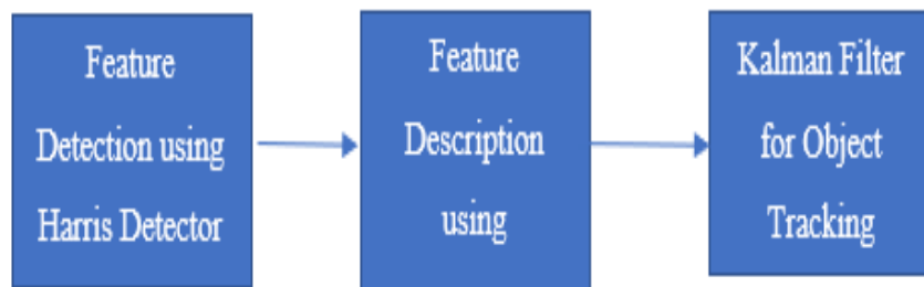
Figure 3.5: Block Diagram for Feature Extraction and Kalman Filtering
