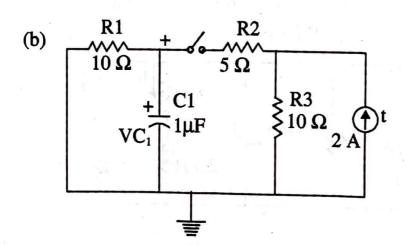
Switch S is closed for infinite time and then opened at t = 0. Find the value of capacitor voltage  $Vc_1$  (t). [C01] [IL] (7.5)
