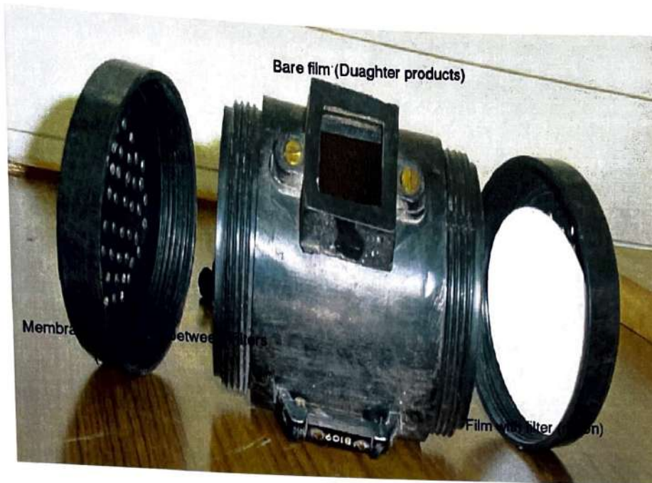
Photograph 3.2: Twin Cup Dosimeter used in Present Study
