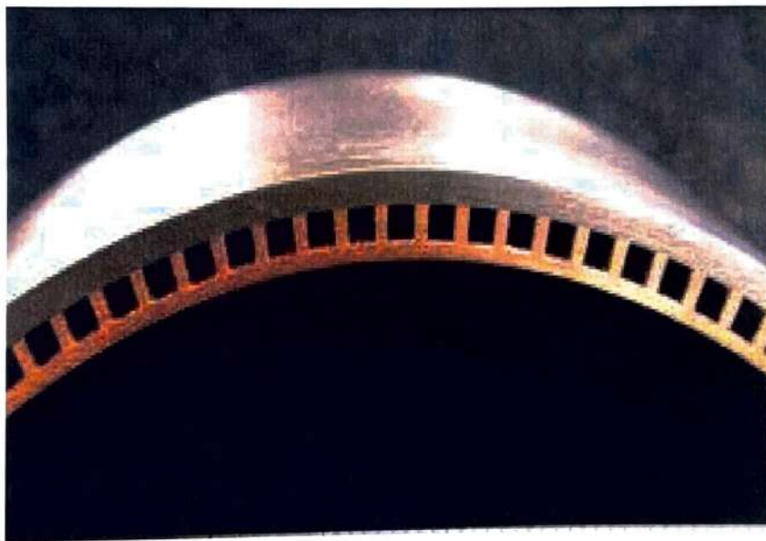
Figure 2.2 : Cut Section of the Electro Plated Combustion Chamber Wall ( http://spl.ch/products/index.html )
