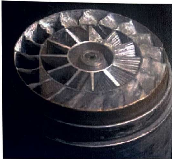
Figure 1.8: Injector with inner and outer Swirlers
