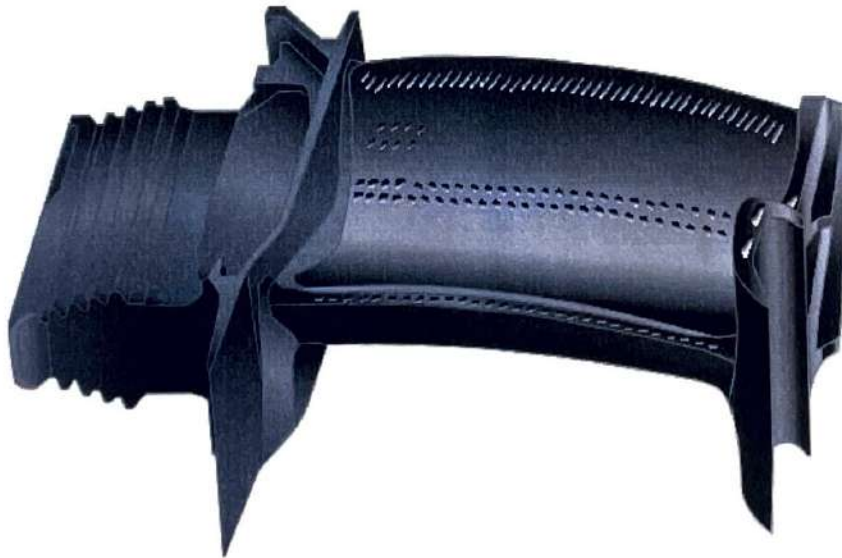
Figure 2.1: Finished Turbine Blade with EDM'd Cooling Holes and Shaped Diffusers ( https://commons.wikimedia.org/wiki/File:GaTurbineBlade.svg )
