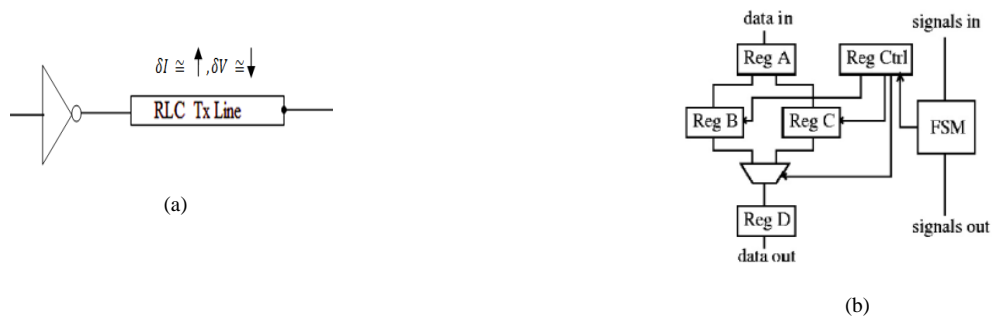
Fig.3.3 Long interconnect lines represented by distributed RLC transmission lines, and driven by (a) An inverter and (b) An architecture of a processor.
