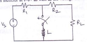
(b) Determine the open circuit and short circuit impedances of the network shown in fig
