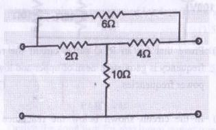
6. (a) Obtain the Thevenin equivalent circuit at terminals B of the active network. (8) CO1
