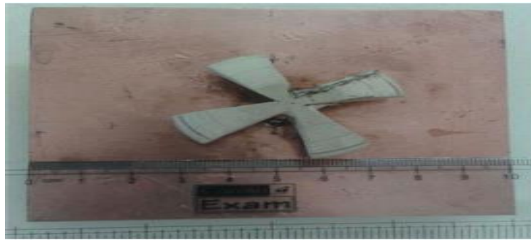
Fig. 2.3.5 Fabricated prototype of antenna [30]
