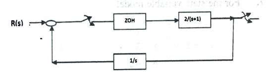
5. A discrete time regulator system has the plant
