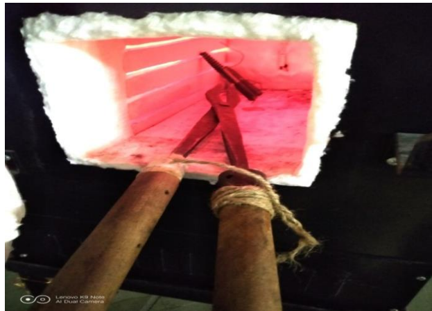
Figure 8.4 Muffle Furnace operating at 860 0 C
