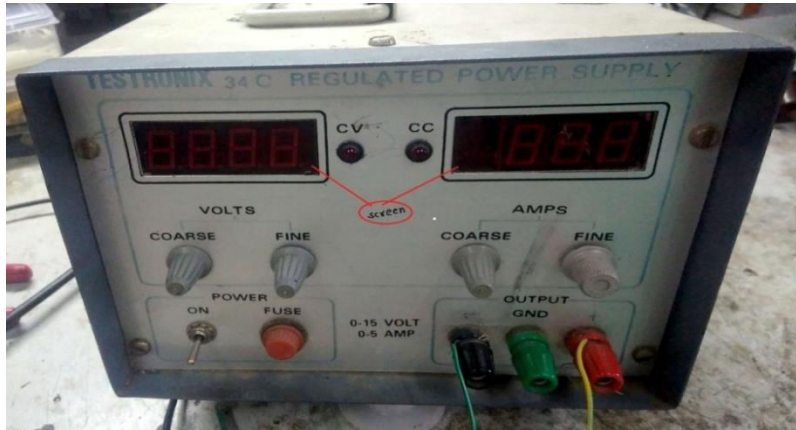
Figure 5.6 DC supply with CV, and CC display
