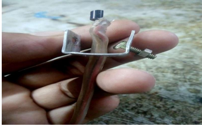
Figure 7.6: Temperature sensor LM35 (with small Al-plate)
