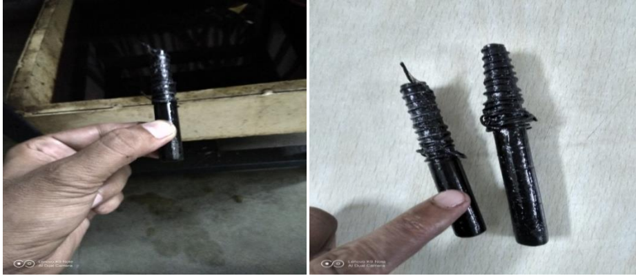
Figure 8.5 Oil-dip tool-fixtures with springs (after quenching)
